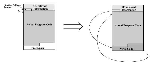
Figure 1: How a Virus Attaches itself to a binary
